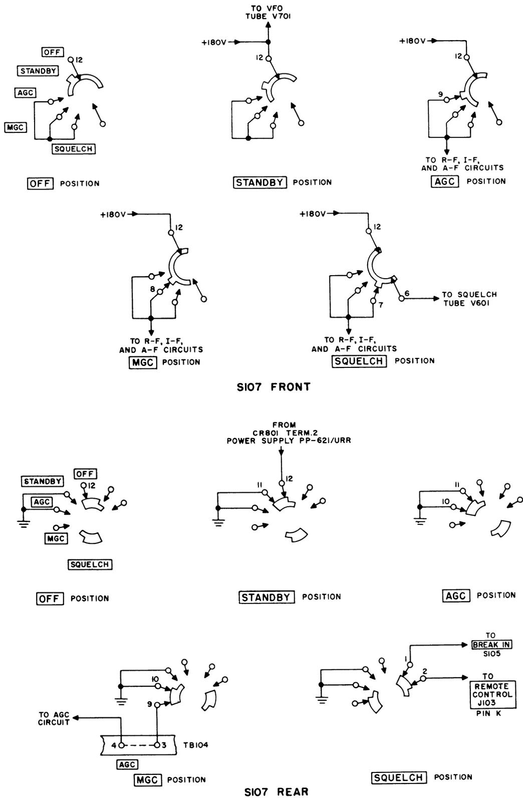
Figure 40. FUNCTION switch, schematic diagram.
