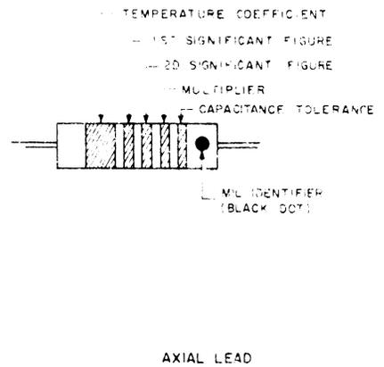
Figure 85. Resistor, inductor, and capacitor color
