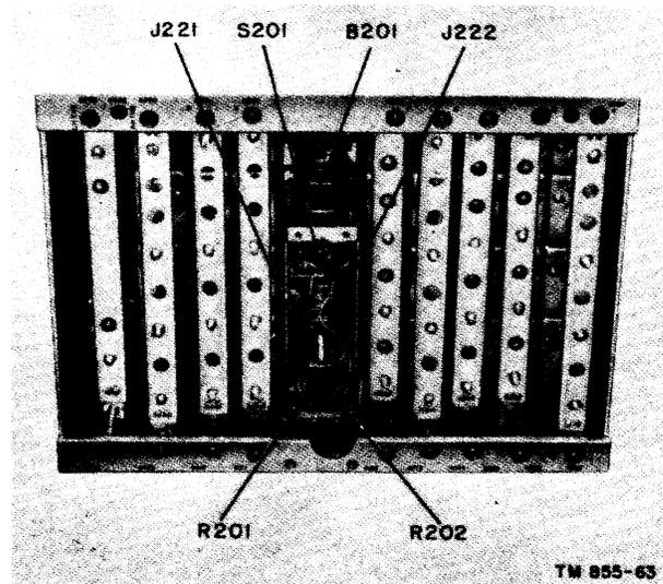
Figure 52. Section of rf subchassis, showing band-switching mechanism.
