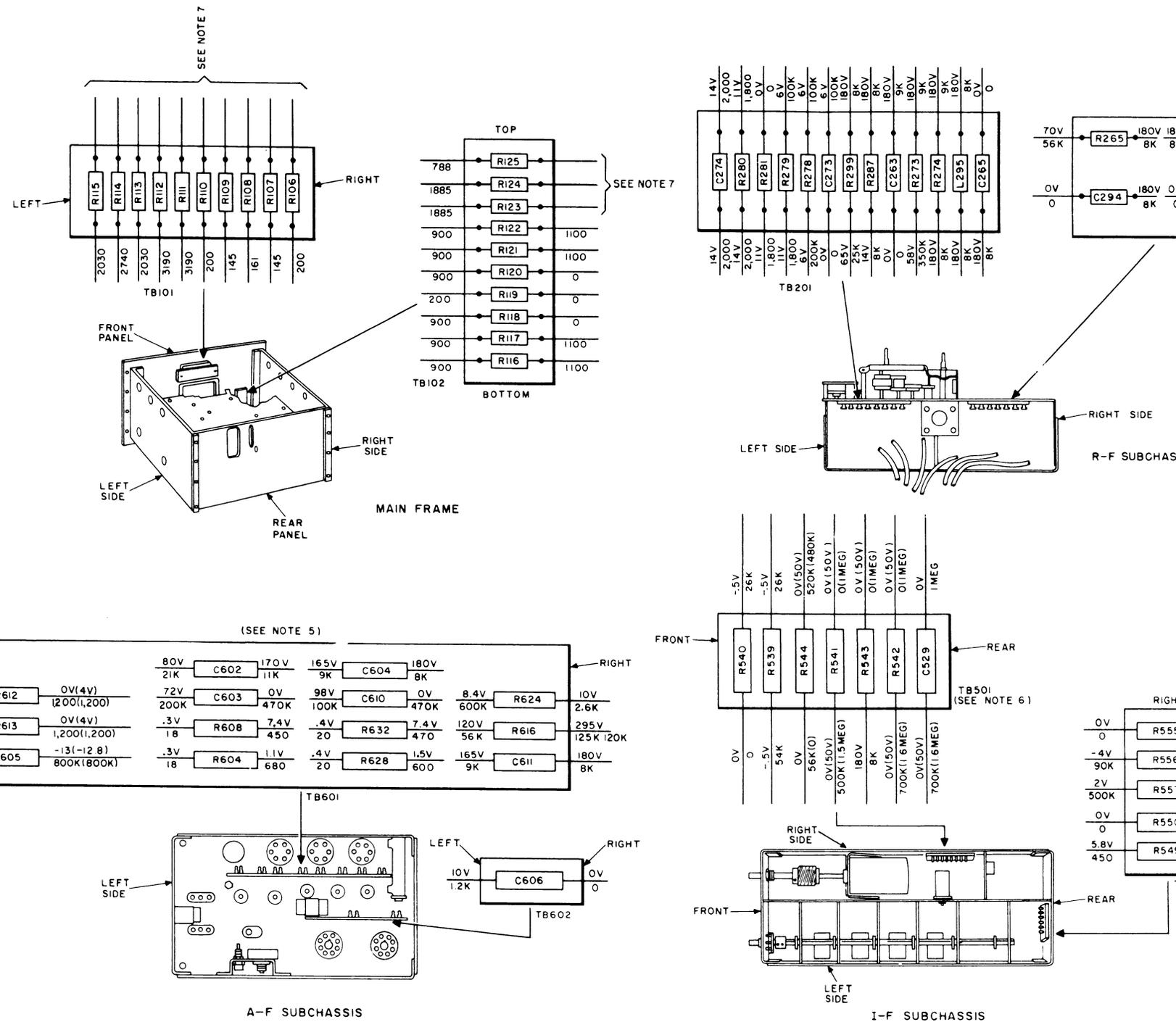
Figure 68. Voltages and resistances at terminal boards.
