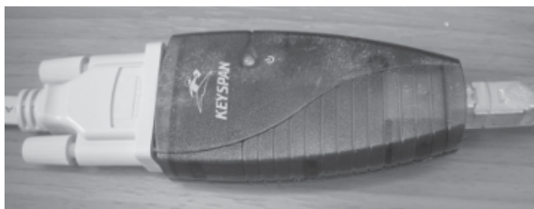
Figure 3-3. A Keyspan serial-to-USB adapter, which can be used to connect a modern laptop or desktop to the serial console of a network device.
