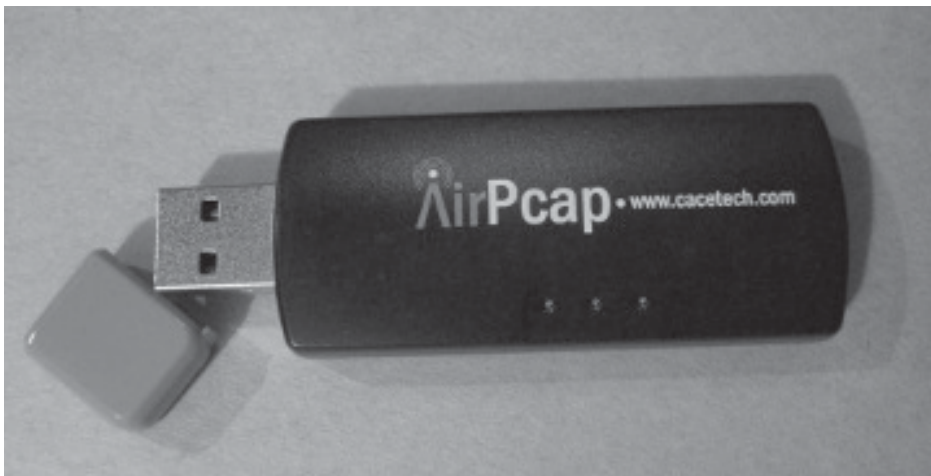
Figure 6–8. The AirPcap USB adapter from Riverbed Technology (previously CACE Technologies).
