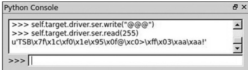
Figure 8-13: Sending @@@ via ChipWhisperer's Python console
