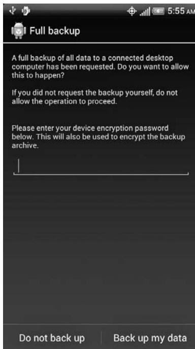
**FIGURE 8-9** Screen activated on a connected Android device when running the ADB backup command
