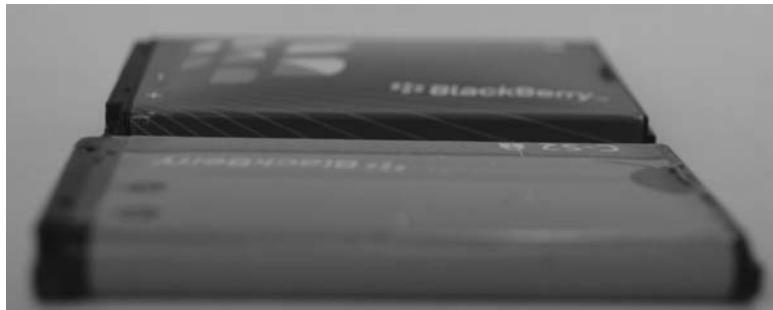
**FIGURE 8-4** A normal battery (front) and a bloated battery (back). The middle of the back battery is distended and could explode, causing damage to the evidence.
