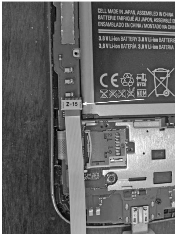
**FIGURE 6-11** Molex connector attached to a Samsung S3 JTAG TAP
