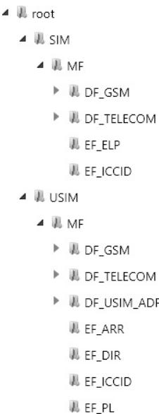
**FIGURE 9-11** File system view of a UICC card and the many folders available to the examiner.
