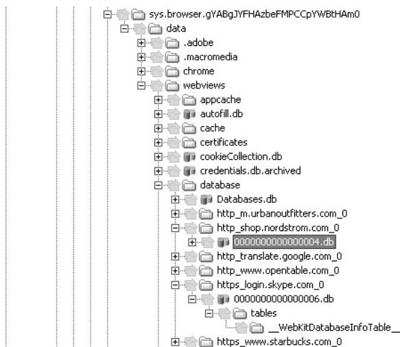
FIGURE 10-21 Navigation into the file system to uncover SQLite databases within the sys.browser application subfolders
