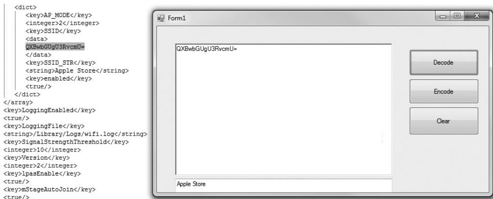
**FIGURE 11-35** Binary Plist com.apple.wifi.plist encodes the SSID values as Base64, which are easily decoded to show the string value.
