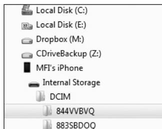
**FIGURE 6-1** File system view of an iOS device connected as a PTP device—Digital Camera Image (DCIM) folder is available
