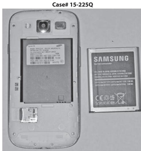
**FIGURE 8-3** The serial numbers of the device should be clearly visible, along with the memory card still in place.
